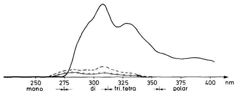
Fig. 4. Synchronous fluorescence spectra with emission wavelength 25 nm higher than that of excitation. Sample: monoaromatic fractions from HPLC. Columns: —, CN; ---,  $\text{NH}_2$ ; ···, silica.
