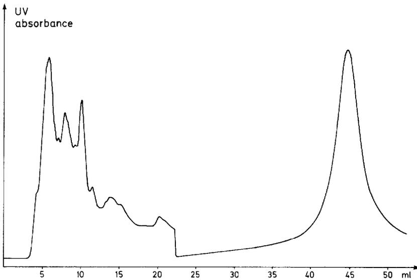
Fig. 2. HPLC of Arabian Light residue on a Waters  $\mu$ Bondapak-NH<sub>2</sub> column, eluted with hexane; flow-rate: 2 ml/min. UV detection at 254 nm. Backflushed at 23.0 ml.
