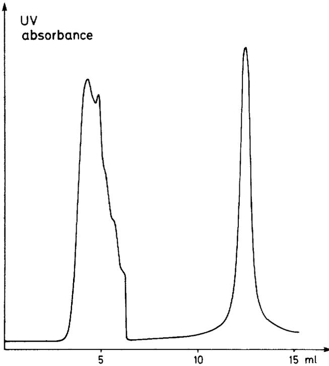
Fig. 1. HPLC of Arabian Light residue on a Waters Rad Pak CN column, eluted with hexane; flow-rate: 1 ml/min. UV detection at 254 nm. Backflushed at 5.9 ml.
