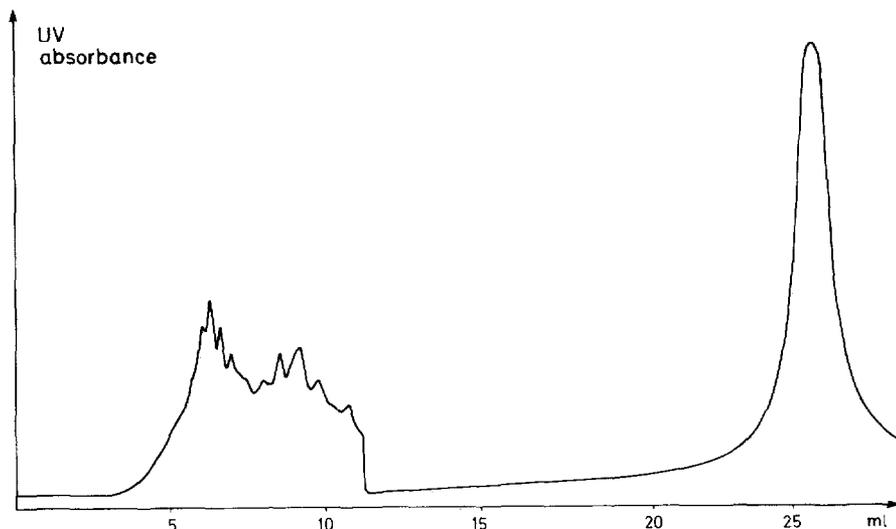
Fig. 3. HPLC of Arabian Light residue on a Waters Rad Pak silica column, eluted with hexane; flow-rate: 1 ml/min. UV detection at 254 nm. Backflushed at 11.5 ml.
